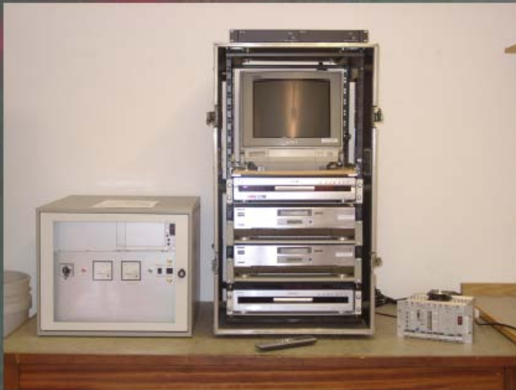
SHRIMP deck components – from l to r: 1500Vac power supply, Recording and monitoring equipment rack, Fibre-optic multiplexer.
