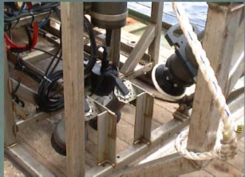
Close-up of the SHRIMP vehicle lighting gantry
